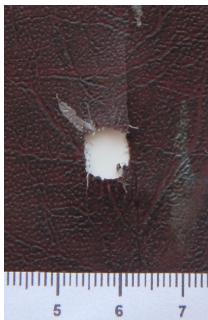
Fig. 5. Damage to the leatherette caused by a shot from Fort 12R at a distance of 25 cm.
