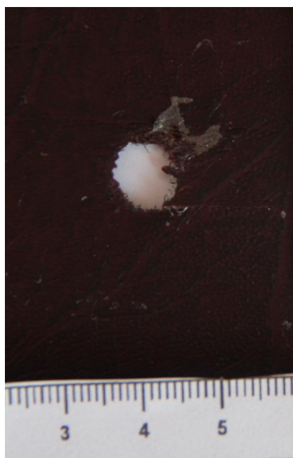
Fig. 3. Damage to the leatherette when shot with the AE790G1 from a distance of 50 cm.
