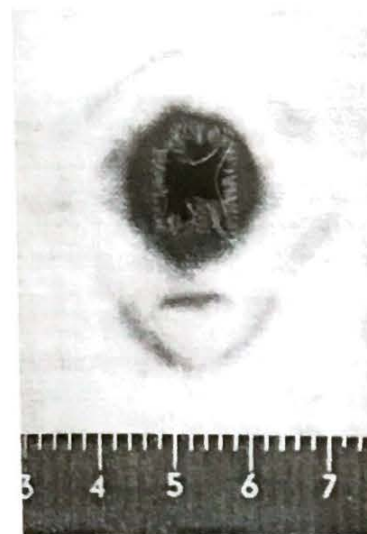
Fig. 2 Damage of target at contact shot
