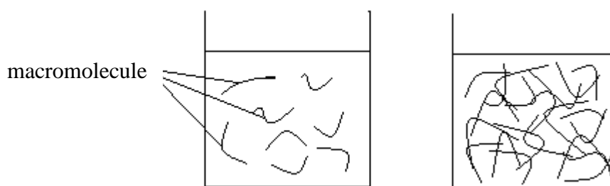
Picture 18.2. Formation a spatial grid at the gelation a - solution of HMC; b - the spatial grid.
