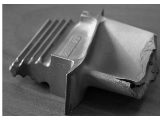
Figure 8 – Destruction of high-pressure turbine blades
