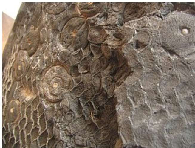
Figure 6 – Thermal ablation protection of the Apollo command module capsule after return
