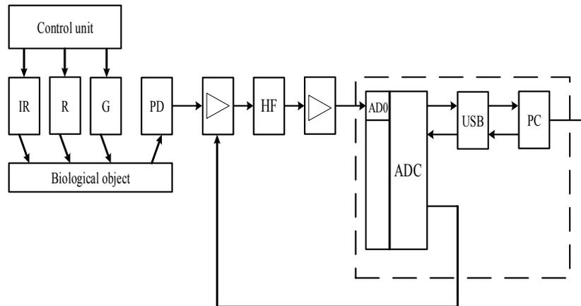
Figure 4. Block diagram of the optical-electronic photoplethysmographic multispectral device for diagnosis of the peripheral blood circulation<sup>31</sup>
