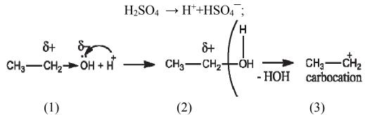
In step (1) the proton attacks the oxygen of hydroxyl group. Further, the proton attached to oxygen, forms the intermediate particle (2), in which oxygen was trivalent, so the water molecule is split off and forms carbocation (3).
