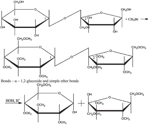
Only  $\alpha - 1,2$ -glucoside bond is under hydrolysis
