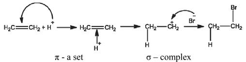
The reaction of alkenes hydrohalogenation used in the synthesis of drugs.
