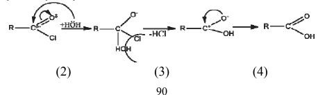
In (1) step attack is a water molecule as a nucleophile on the carbonyl carbon. Dual carbon-oxygen bond is broken and the water joins (2). Water is pushed out of the particle (2) chloride - anion and a proton simultaneously cleaved from the molecule of water, as water becomes trivalent oxygen as a result of accession. Formed an intermediate particle (3), in which there is a redistribution of electron density, and form the final product (4) carboxylic acid.
