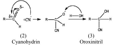
In step (1) cyanide-anion as the nucleophile attacks the carbon of the aldehyde group. As a result, it breaks the double bond carbon-oxygen, and cyanide-ion associates (2), with the formation of an intermediate particle with negative charge on oxygen, which is neutralized by a proton from a water molecule (water easily dissociates under the action of the negative charge of oxygen, that is, **water is the protonation**, which is produced by the final product - **a cyanohydrin**.
