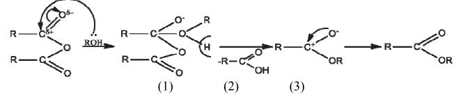
(4) In step (1) attack is a molecule of alcohol as a nucleophile on the carbonyl carbon. Dual carbon-oxygen bond is broken and alcohol joins (2). Alcohol pushes the particles of (2) of the carboxylate anion and a proton simultaneously cleaved from the molecule of alcohol, as oxygen becomes trivalent in the result of a merger. In the intermediate particle (3), is the redistribution of electron density, and form the final product (4) - ester.
