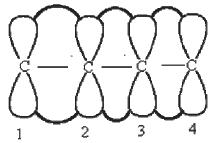
P-orbitals, which form a  $\pi$ -bond, are also called  $\pi$ -orbitals or  $\pi$ -electron density;  $\pi$ -electron density is located in space, so it is very mobile and is over lapped between the C<sub>2</sub> -C<sub>3</sub>
