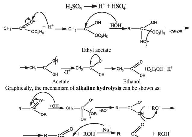
Hydroxide ion, which is the catalyst that attacks the carbon atom of the carboxyl group (1). As a result, the intermediate particle (2), in which the hydroxyl group of associates and pushes alkoxy RO<sup>-</sup>. Formed particle (3), from which the proton is split off and goes to the alkoxy group. As a result of redistribution of electron density occurs
