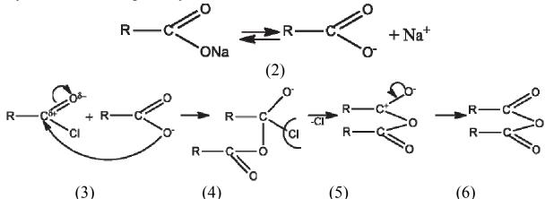
Salt of the carboxylic acid (1) dissociates and forms carboxylate-anion (2), which is the nucleophile. Further, the carbon halide (3) is attacked by a nucleophile (2). As a result of this attack breaks the double bond C=O, and the nucleophile associates (5). Then cleaved from the carbon chloride-anion formed by the intermediate particle (6), which is the redistribution of electron density, resulting in a final product - **anhydride** (7).
