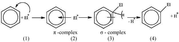
The scheme of the mechanism of electrophilic substitution:
