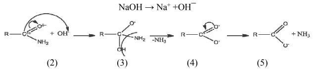
In (1) step is an attack OH - anion as the nucleophile on carbon oxo - group. Dual carbon-oxygen bond is broken and formed anion (2), which split off from both the amino group and a proton, forming a molecule of ammonia. In the intermediate particle (3) are the redistribution of electron density and the formation of end products - the carboxylate anion (4) and the ammonia molecule (5).
