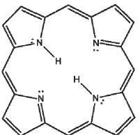
The conjunction is a porfin system and consists of 26 p-electrons. Energy delocalization of nucleus: 840 kJ / mol.
