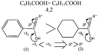
Aromatic acids are stronger than acid - derived cycloalkanes, as a positive inductive effect  $s\rho^2$ - hybrid carbon benzene ring (+I<sub>1</sub>) is less than the positive inductive effect  $s\rho^3$ -hybrid carbon atoms of cyclohexane (+I<sub>2</sub>), so  $\delta$ +>' $\delta$ +; here fore increases displacement of unshared electron pairs from oxygen to carbon (1), i.e. on the oxygen atom decreases the electron density and the proton is split off more easily.
