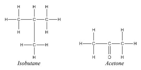
**b)** Properties of materials depend not only on the qualitative and quantitative composition, but also on the order in which the atoms are combined in the molecule, i.e the chemical structure of the molecule:
