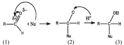
In step (1) the nucleophile attacks the carbon atom due to the lack of electron density. As a result of the attack, it breaks the double bond, nucleophile attached to the carbon and forms the intermediate particle (2). The negative charge on oxygen in the particle (2) neutralizes the electrophile (usually a proton  $H^+$ ), and produces the final product of the reaction (3).
