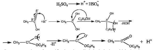
Reverse reaction of esterification is called hydrolysis, which is also on the mechanism of nucleophilic substitution. Hydrolysis can proceed in acidic and alkaline media.
