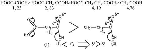
Dibasic acid is stronger than monobasic, since the second carboxyl group pulls itself from the radical electron density and its inductive effect (I<sub>1</sub>) becomes smaller, so that  $\delta$ +>'  $\delta$ + thereby increasing the displacement of the unshared electron pair of oxygen to carbon (1), i.e. on the oxygen atom decreases the electron density and the proton is split off more easily.
