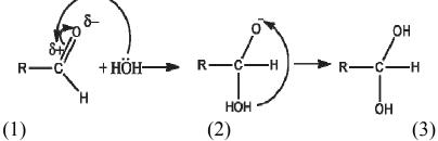
The first is the attack of a water molecule as the nucleophile (1), and to form an intermediate compound (2), in which the oxygen in the aldehyde of the negative charge arises, and in the water molecule appears trivalent oxygen, which is impossible. Therefore, water molecules are split off from the proton and move to the negatively charged oxygen (2). This is a finished product result (3).
