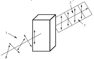
If the path of the polarized beam is to be put in a tube with a solution of an organic compound, the plane of polarization (4) will rotate to the right or to the left.
