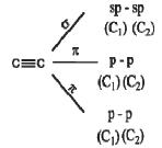
C-H bond in the alkyne is the  $\sigma$ -bond that is formed by the overlapping of sp-hybrid orbitals of carbon and s-orbitals of the hydrogen atom.
