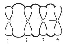
That is, the electron density is not centered between two adjacent carbon atoms and is **delocalized** over the whole system (i.e. molecule) and formed by a single dual of four central clouds that cover all carbon atoms:
