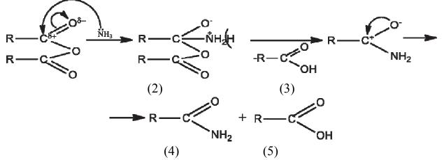
In (1) step attack is a molecule of ammonia as a nucleophile on the carbonyl carbon dioxide. Dual carbon-oxygen bond is broken and ammonia joins (2). Ammonia is pushed out of the particle (2) carboxylate - anion and a proton simultaneously cleaved from the molecule of ammonia, as nitrogen is tetravalent with the accession (from the positive
